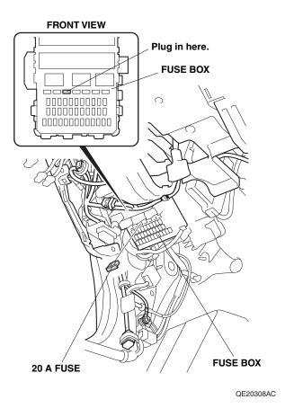
47. Using isopropyl alcohol on a shop towel, thoroughly clean the area where the fuse label will attach.
