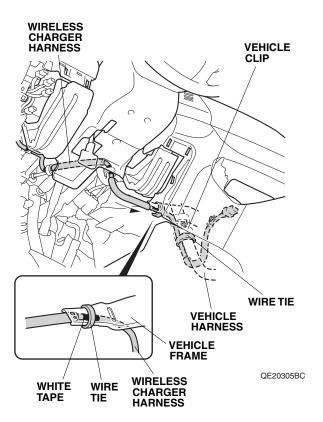
43. Secure the wireless charger harness to the vehicle harness with one wire tie.
