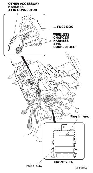
30. Plug the remaining wireless charger harness 4-pin connector into the fuse box.
