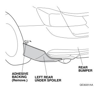
19. Using your hand, firmly press the left rear under spoiler against the rear bumper for 30 seconds.
