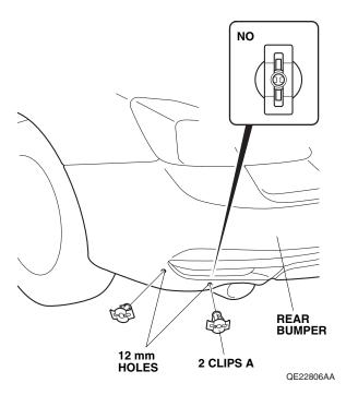
12. Thread a self-tapping screw into each pierced mark to make two holes in the rear bumper. Remove the self-tapping screw.
