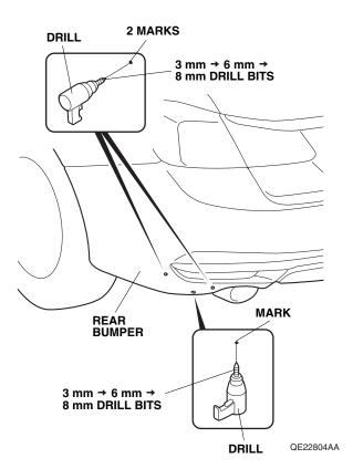
9. Enlarge the two upper holes to 12 mm using a 12 mm drill bit. Remove any burrs.
