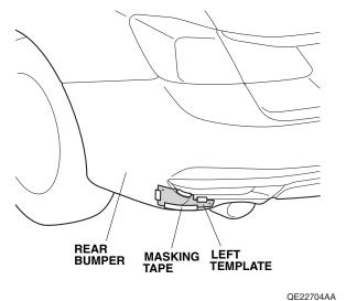
5. Using a pushpin, pierce the rear bumper through the hole in the template and dimple. Remove the template.
