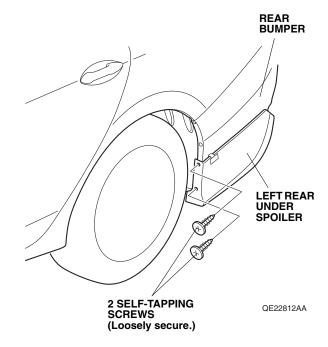
While applying light pressure against the left rear under spoiler, carefully remove the adhesive backing.
