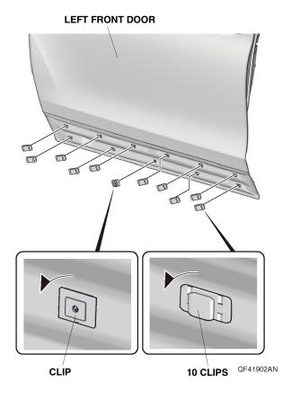
Reinstall the 11 clips removed in step 3 and one screw removed in step 1 to the left front door lower trim.
