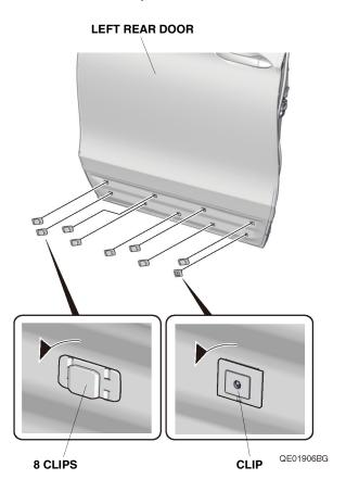
Reinstall the nine clips removed in step 16 and one screw removed in step 14 to the left rear door lower trim.
