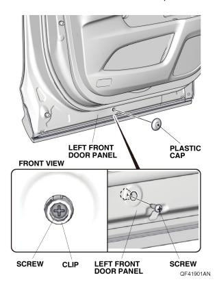
2. Slide and remove the left front door lower trim from the left front door.
