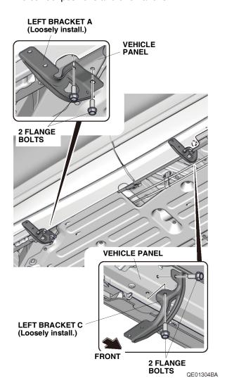
4. With the help of an assistant, install the left running board to the left bracket A and left bracket C with four flange bolts. Torque the flange bolts to 27 N·m (20 lb·ft).
