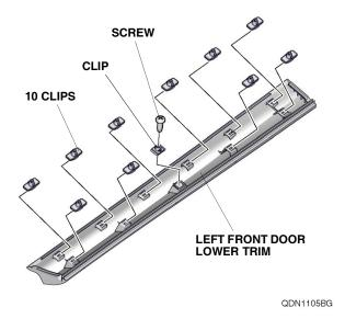
Attach masking tape to the left front door lower trim as shown.
