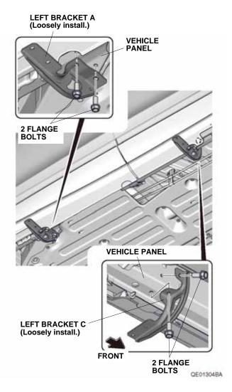
4. With the help of an assistant, install the left running board to the left bracket A and left bracket C with four flange bolts. Torque the flange bolts to 27 N·m (20 lb·ft).
