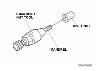
22. Insert the rivet nut into the hole in the trailer hitch and insert the hex wrench in the 6 mm rivet nut tool. NOTE: Rivet nut may be a tight fit into the vehicle hole. If they do not slide in easily, use a hammer to tap them into place.
