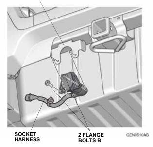
28. Remove the dummy connector from the vehicle 10-pin connector. Plug the socket harness 10-pin connector into the vehicle 10-pin connector. NOTE: Removal of the vehicle 10-pin connector from the vehicle clip may be necessary.
