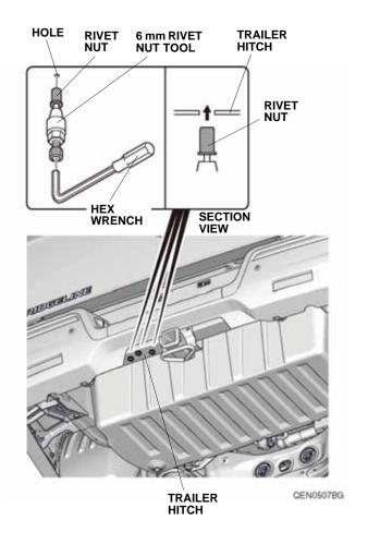
23. While holding the 6 mm rivet nut tool with the hex wrench, turn the 19 mm open end wrench counterclockwise and install the rivet nut to the trailer hitch.
