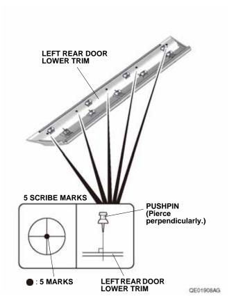
While wearing eye protection, drill the five pierced marks to 7 mm. Drill first with a 3 mm drill bit, then finish with a 7 mm drill bit. Remove any burrs. NOTE: Make sure to drill perpendicularly to the left rear door lower trim.
