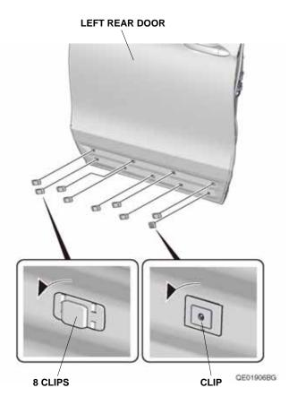
17. Reinstall the nine clips removed in step 16 and one screw removed in step 14 to the left rear door lower trim.
