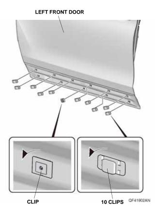
Reinstall the 11 clips removed in step 3 and one 4. screw removed in step 1 to the left front door lower trim.
