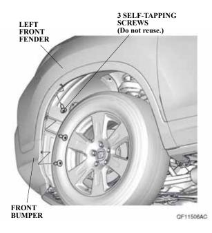
3. Install the three snap-screws and three washers on the front bumper.
