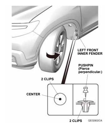
Using a pushpin, pierce the center of the top two clips on the left front inner fender.
