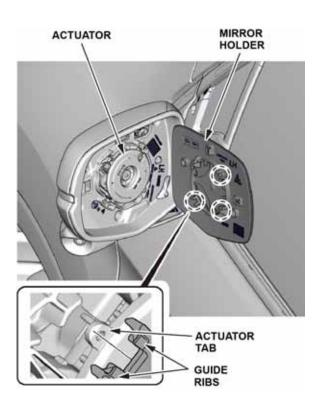
4. Move the mirror holder in all directions to confirm it is installed securely.
