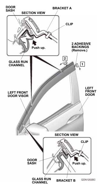
Using a soft towel, press and hold the left front door visor against the door sash for 30 seconds.
