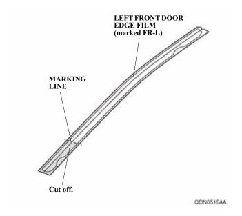
8. Open the left front door again. Peel back about 50 mm (1.97 in.) of adhesive backing from the left front door edge film. Line up the V-notch in the left front door edge film with the character line of the left front door.
