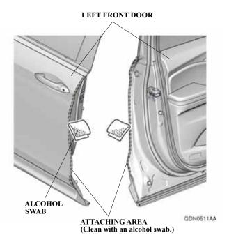
4. Close the left front and rear doors. Using a spray bottle with 3M protective tape application solution, spray the area where the left front door edge film will attach.
