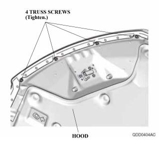
11. Using an alcohol swab, clean inside the hood where the advice label will attach.
