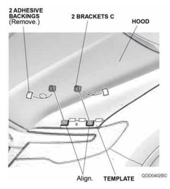
8. Turn the template over and repeat steps 5 through 7 to install the other two brackets C on the right side of the vehicle.
