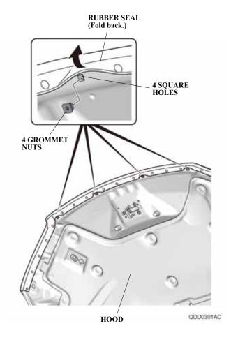
2. Fold back the rubber seal, and using an alcohol swab, clean the areas of the hood where the two brackets A and the two brackets B will mount.
