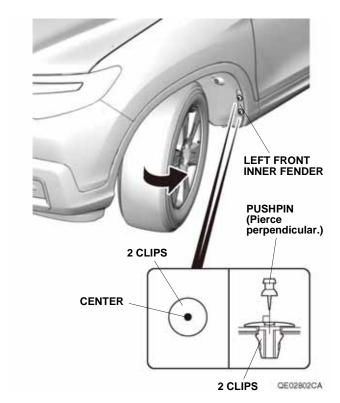
2. Using a pushpin, pierce the center of the top two clips on the left front inner fender. NOTE: Make sure to pierce perpendicular to the left front inner fender.
