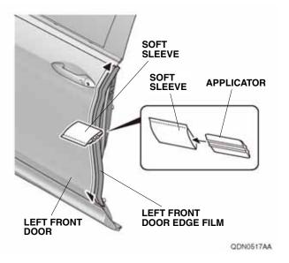
11. Slowly remove the protective film from the left front door edge film.
