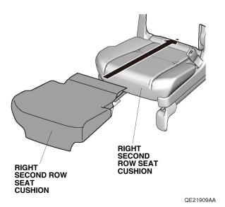
7. Secure the three hooks and fasteners to the right second row seat cushion. Insert one tab to the right second row seat cushion.
