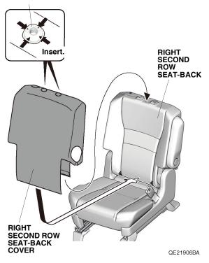
Secure the right second row seat-back cover with the fasteners.
