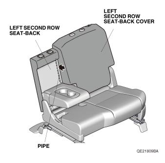
10. Secure the left second row seat-back cover with the fasteners.
