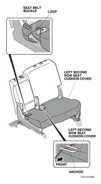
Secure the left second row seat cushion cover with the fasteners. NOTE: Do not cover the anchor labels.
