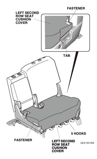
15. Install the seat belt buckle into the loop as shown. Insert the left second row seat cushion cover under the anchor.
