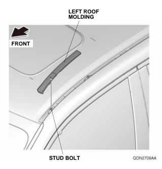
If the roof molding is equipped with a plastic cap, go to step 12; otherwise, go to step 14.
