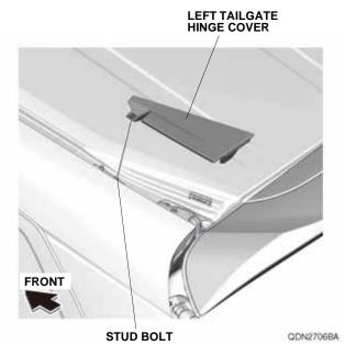
8. Open the tailgate. Install the left tailgate hinge cover extension to the left tailgate hinge cover with one clip and one pin.
