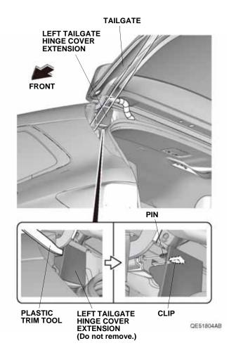
Close the tailgate halfway. Gently pry up on the rear edge of the left tailgate hinge cover, and remove it as shown. Do not reuse the left tailgate hinge cover.
