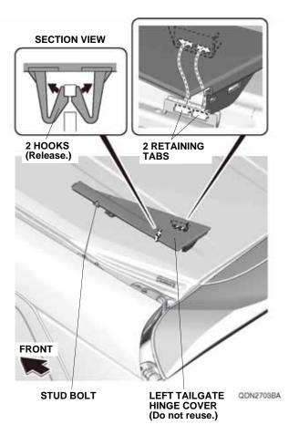
6. Remove the two clips from the two stud bolts on the roof.
