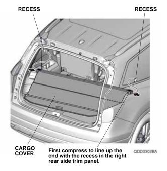
4. Attach each hook of the cargo cover to the headrestraint stay.
