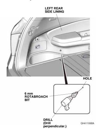
10. Install one rivet into the hole on the left rear side lining as shown.
