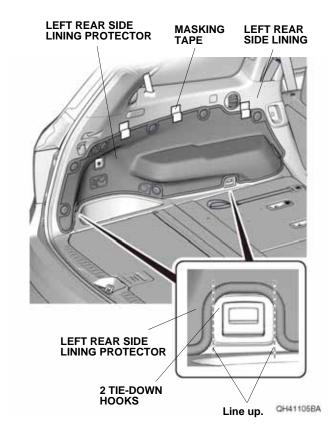
6. Using a T-pin, pierce the left rear side lining through the hole in the snap No.1 as shown. Remove the masking tape from this snap attached in step 3. NOTE: Make sure to pierce the left rear side lining perpendicular. Do not remove the masking tape from the other snaps at this time.
