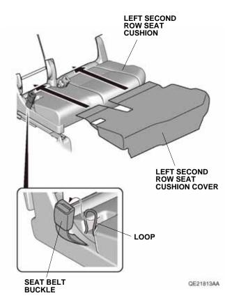
14. Secure the left second row seat cushion cover with the five hooks, one tab, and the fasteners.
