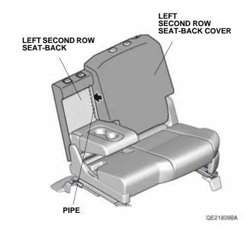
Secure the left second row seat-back cover with the fasteners.
