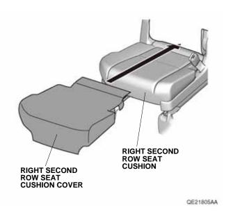
6. Secure the three hooks and fasteners to the right second row seat cushion. Insert one tab to the right second row seat cushion.
