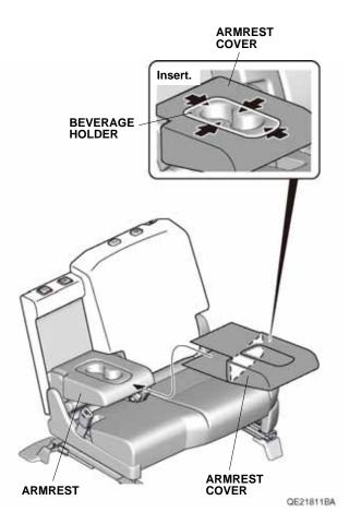
12. Raise the armrest. Pull out the armrest cover between the armrest and left second row seat-back, and secure the armrest cover with the fasteners.
