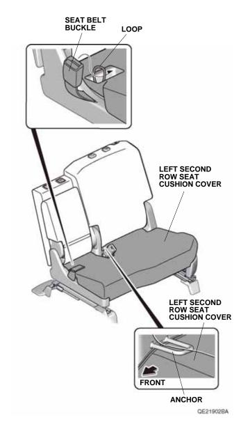
16. Secure the left second row seat cushion cover with the fasteners.
