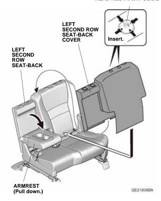
9. Insert the pipe into the left second row seat-back.
