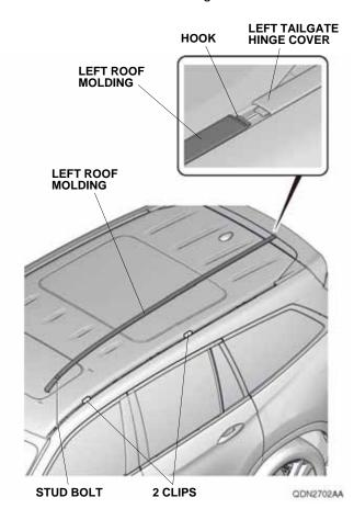
Open the tailgate. Using a plastic trim tool, release the left tailgate hinge cover extension as shown. NOTE: Do not remove the tailgate hinge cover extension.
