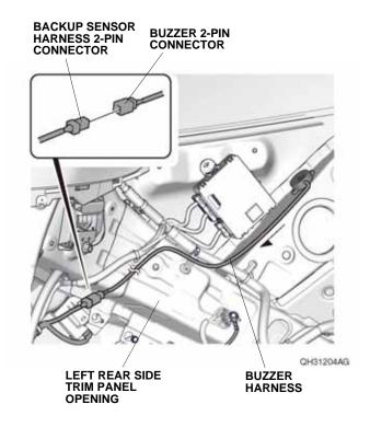
35. Bundle up the excess buzzer harness, and secure it and the 2-pin connectors to the vehicle harness with three wire ties as shown.
