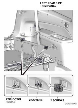
12. Using a plastic trim tool, pull the cover and remove the cargo hook.
