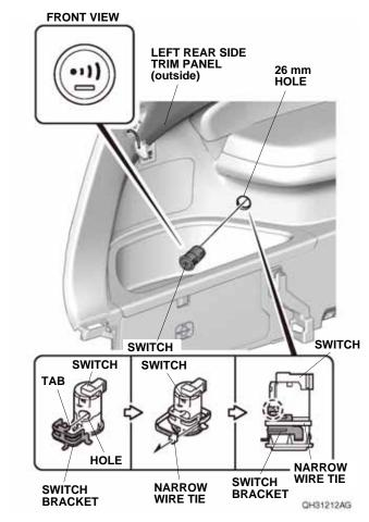
48. Line up the tab on the switch bracket with the hole on the switch and secure the switch bracket to the switch with one narrow wire tie.
