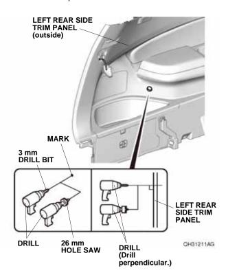
47. Install the switch into the 26 mm hole.
