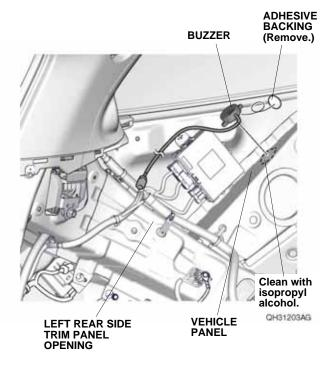
33. Remove the adhesive backing from the buzzer and attach the buzzer to the vehicle panel as shown.
