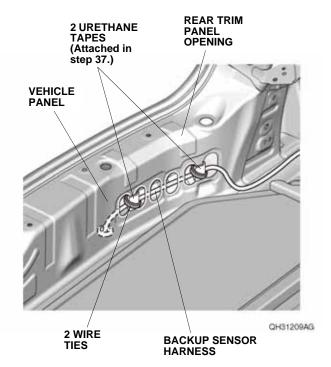
41. Using isopropyl alcohol on a shop towel, thoroughly clean the vehicle panel where the aluminum tape will attach.
