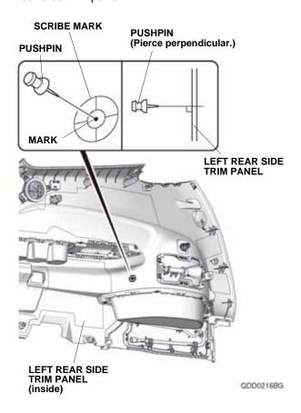
46. While wearing eye protection, drill the pierced mark on the left rear side trim panel using a 3 mm drill bit. Enlarge the 3 mm hole to 26 mm using a 26 mm hole saw, and remove any burrs.
