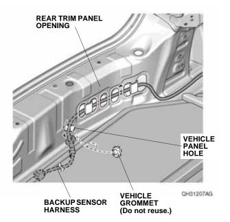
39. Secure the grommet on the backup sensor harness to the vehicle panel hole.
