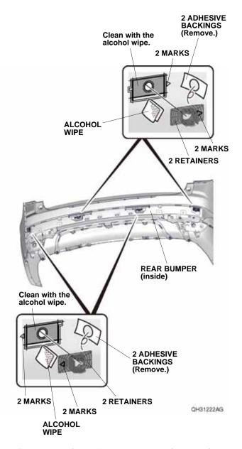
62. Remove the four adhesive backings from the four retainers, and attach the four retainers to the rear bumper as shown.
