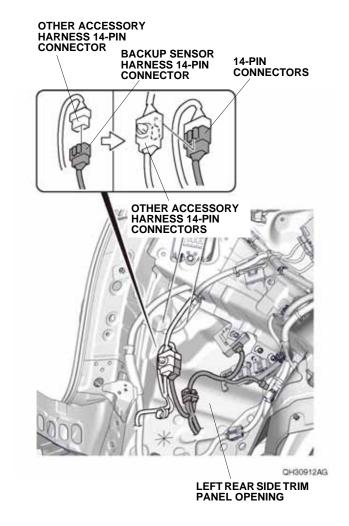
29. Install the 14-pin connectors to the other accessory harness 14-pin connectors as shown.
