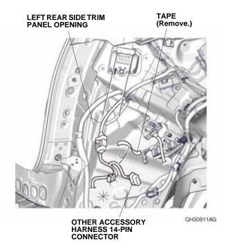
28. Plug the other accessory harness 14-pin connector into the backup sensor harness 14-pin connector.
