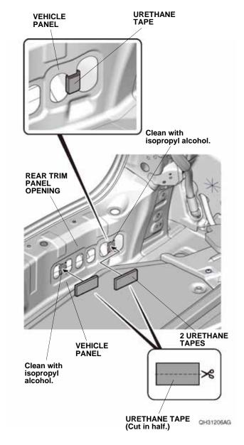
37. Using scissors, cut one urethane tape in half, and attach the two pieces to the vehicle panel as shown.
