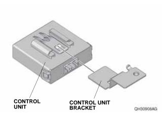
24. Install the control unit to the vehicle panel with one flange bolt as shown.
