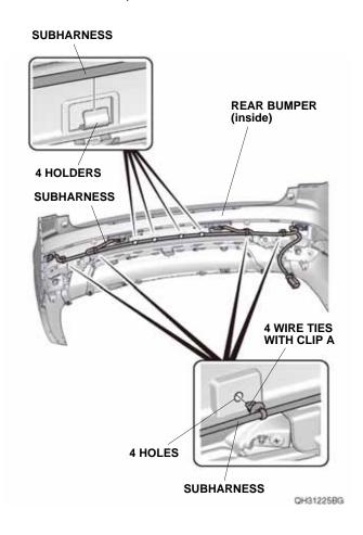
66. With the help of an assistant, bring the rear bumper close to the vehicle, and plug the subharness 4-pin connector into the backup sensor harness 4-pin connector. Install the rear bumper.
