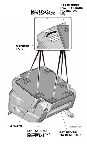
25. Using a pushpin, pierce the left second row seatback through the hole on the left second row seatback protector snap as shown. Remove the masking tape attached in step 20 from the left second row seat-back protector.
