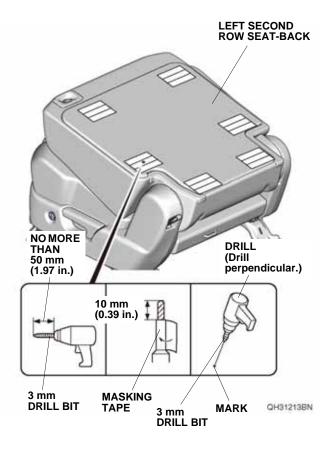
28. While wearing eye protection, use a 8 mm Rotabroach bit to drill the hole as shown. Remove any burrs.
