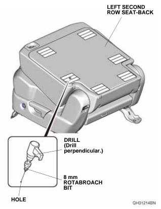
29. Remove the masking tape attached in step 24 at the drilled position from the left second row seat-back. NOTE: Do not remove the masking tape where the left second row seat-back is not marked yet.
