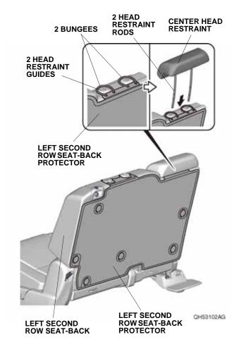
19. Install the head restraint on the left second row seat.
