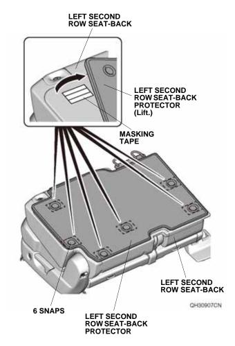
Using a pushpin, pierce the left second row seatback through the hole on the left second row seatback protector snap as shown. Remove the masking tape attached in step 2 from the left second row seatback protector.
