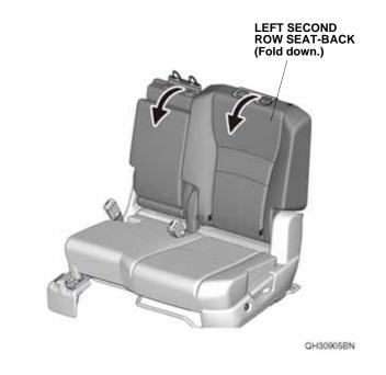
4. Place the left second row seat-back protector on the left second row seat-back. Secure the two head restraint holders to the four head restraint guides as shown.
