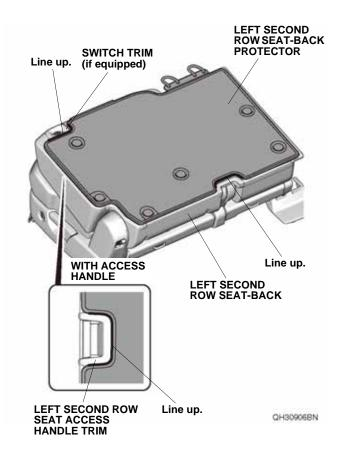
6. Lift the left second row seat-back protector, and attach masking tape to the left second row seat-back where the snaps will be located.
