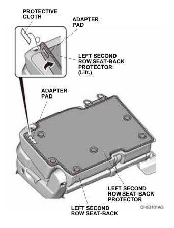
17. Apply pressure to the left second row seat-back protector at the area were the Velcro is located, make front to back movements while applying pressure to ensure proper attachment of adapter pad. 18. Raise the left second row seat-back. Install the center head restraint on the left second row seat. Bungee on center head restraint should be installed at this point, making sure it is secure by the head restraining rods.
