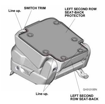
24. Lift the left second row seat-back protector, and attach masking tape to the left second row seat-back where the snaps will be located.
