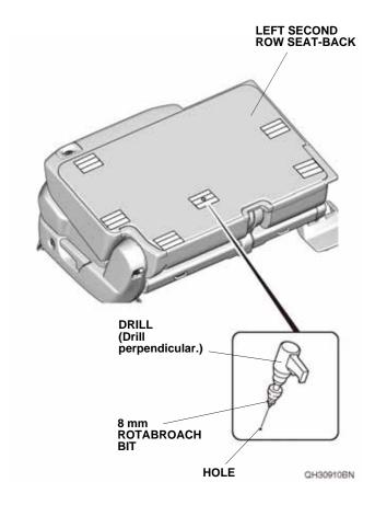
11. Remove the masking tape attached in step 6 at the drilled position from the left second row seat-back. NOTE: Do not remove the masking tape where the left second row seat-back is not marked yet. 12. Install the snap, and well nut into the hole on the left second row seat-back with one screw as shown.
