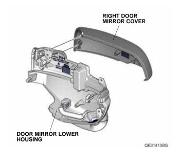
9. Secure the right door mirror cover with the TORX screw removed in step 6.
