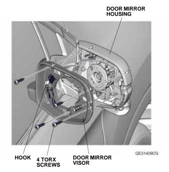
5. Using needle nose pliers wrapped with tape, remove the door mirror housing, and unplug the vehicle connectors.
