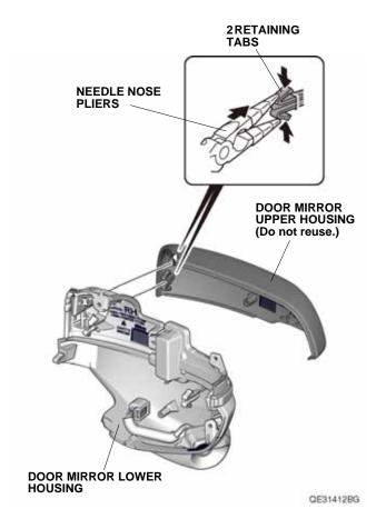
8. Install the right door mirror cover on the door mirror lower housing.
