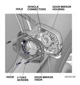
13. Plug the vehicle connectors into the mirror holder.
