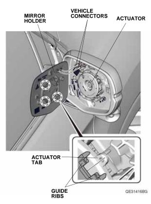
Align the guide ribs on the mirror holder so they line up on each side with the actuator tabs. Reinstall the mirror holder on the actuator. 15. Move the mirror holder in all directions to confirm it is installed securely.
