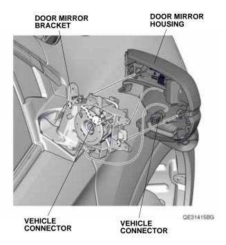
Install the door mirror housing on the door mirror bracket.
