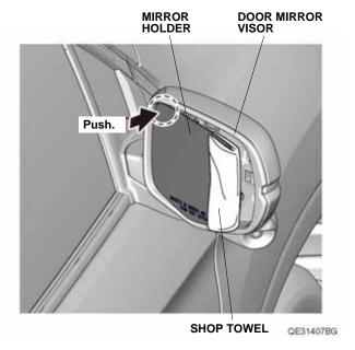
Remove the mirror holder, and unplug the vehicle connectors.
