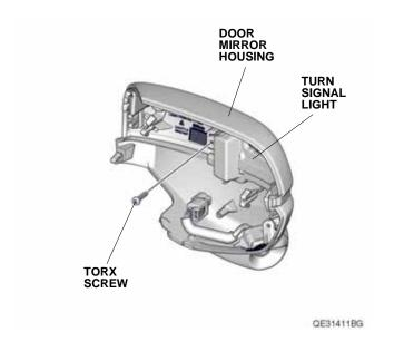
7. Using the needle nose pliers, remove the door mirror upper housing.
