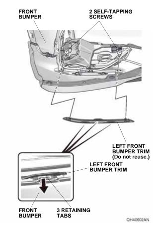
Install the new left front bumper trim to the front bumper with two self-tapping screws and three retaining tabs.
