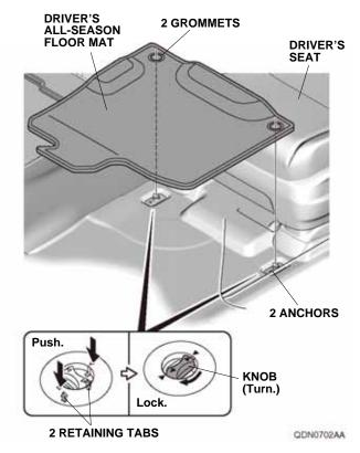
Place the grommets in the driver's all-season floor mat over the anchors. Push the grommets into the anchors to secure the retaining tabs, then turn the knobs 90° to secure the driver's all-season floor mat.  Place the grommets in the passenger's all-season floor mat over the anchors. Push the grommets into the anchors to secure the retaining tabs, then turn the knobs 90° to secure the passenger's all-season floor mat.
