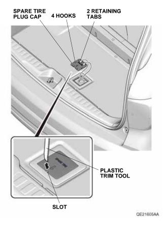
3. Remove the spare tire plug to access the spare tire hoist shaft. Lower the spare tire completely.
