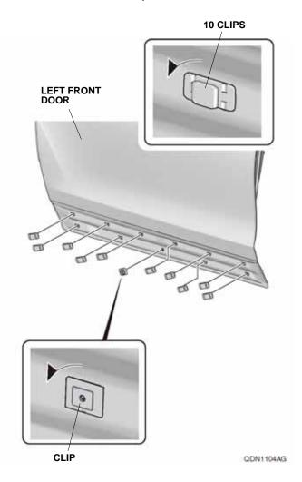
4. Reinstall the eleven clips removed in step 3 and one screw removed in step 1 to the left front door lower trim.
