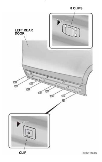
17. Install the nine clips removed in step 16 and the screw removed in step 14 to the left rear door lower trim.
