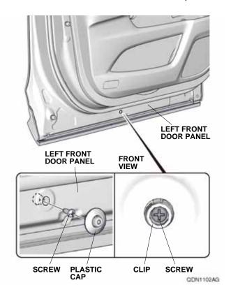
2. Slide the left front door lower trim, and remove the left front door lower trim.
