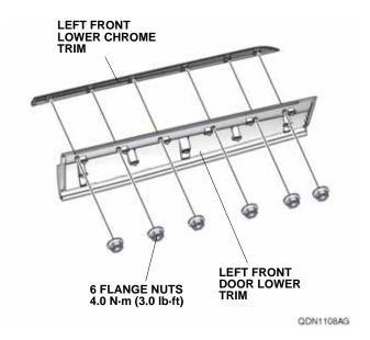
10. Secure the left front lower chrome trim to the left front door lower trim with six flange nuts. Torque the flange nut to 4.0 N·m (3.0 lb·ft)
