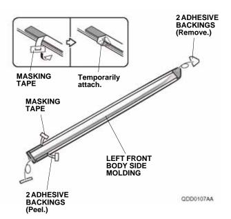
7. Line up the left front body side molding with the front and middle templates, and attach it to the left front door as shown.
