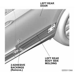
13. Using a rubber roller, apply firm pressure against the left rear body side molding and roll from one end to the other. Apply firm pressure especially at the ends.
