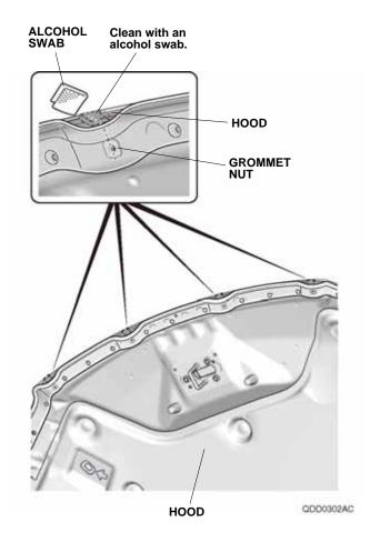
Remove the four adhesive backings from the four protection films, and attach them to the front of the hood area where the two brackets A and the two brackets B will mount.
