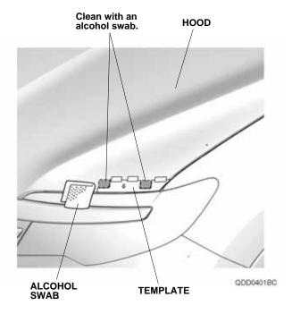
7. Remove the two adhesive backings from the two brackets C, and line up with the template secured in step 5. Remove the template.
