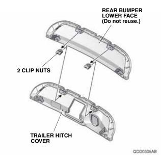
6. Install the trailer hitch cover to the rear bumper with six retaining tabs, two clips, two self-tapping screws, and two bolts removed in step 4.
