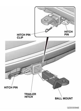
After the first 600 miles (1,000 km) of towing, have your Honda Dealer re-check the tightness of the trailer hitch bolts.
