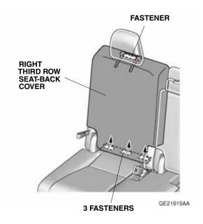
5. Secure the right third row seat-back cover with the fastener. Secure the strap to the right third row seat-back cover with the fastener.
