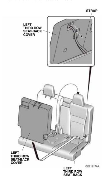
Secure the left third row seat-back cover with the fasteners.
