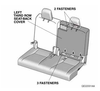
8. Secure the left third row seat-back cover with the fastener. Secure the strap to the left third row seat-back cover with the fastener.
