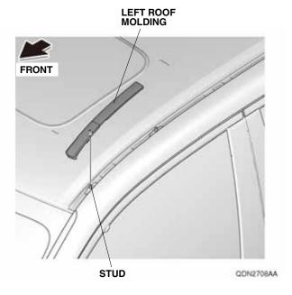
Install the left roof rail base to the three stud bolts with three 6 mm TORX nuts. Make sure the roof rail base is installed in the correct position. Torque the 6 mm TORX nuts to 6.9 - 11.8 N·m (5.1 - 9 lb·ft).
