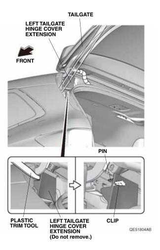
3. Close the tailgate halfway. Gently pry up on the rear edge of the left tailgate hinge cover. Do not reuse the left tailgate hinge cover.
