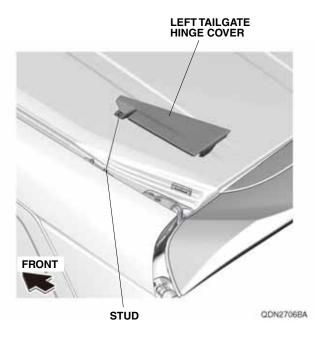
6. Open the tailgate. Install the left tailgate hinge cover extension on the left tailgate hinge cover with one clip and one pin.
