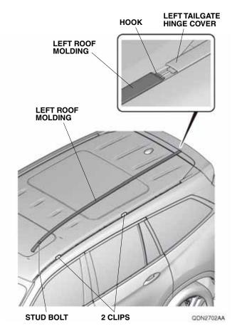
Open the tailgate. Using a plastic trim tool, release the left tailgate hinge cover extension. NOTE: Do not remove the tailgate hinge cover extension.
