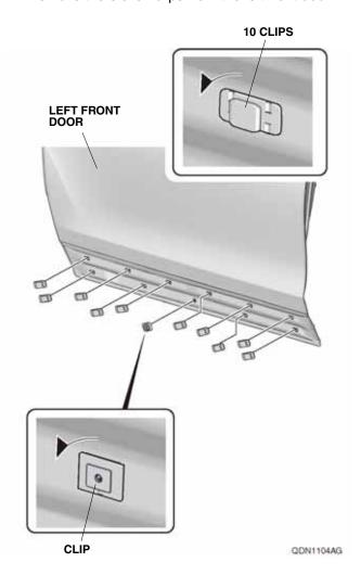
Reinstall the eleven clips removed in step 3 and one screw removed in step 1 to the left front door lower trim.
