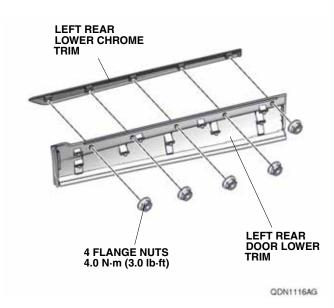
23. Secure the left rear lower chrome trim to the left rear door lower trim with five flange nuts. Torque the flange nut to 4.0 N·m (3.0 lb·ft)
