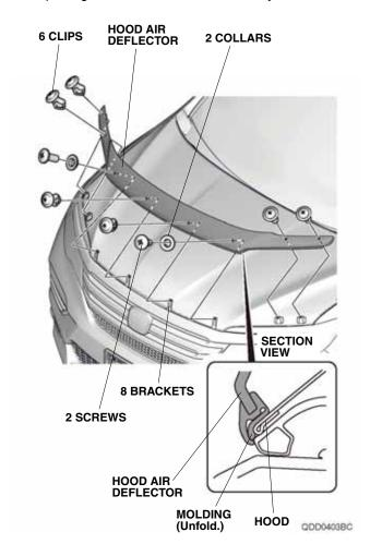
10. Open the hood. Tighten the four truss screws loosely installed in step 4.
