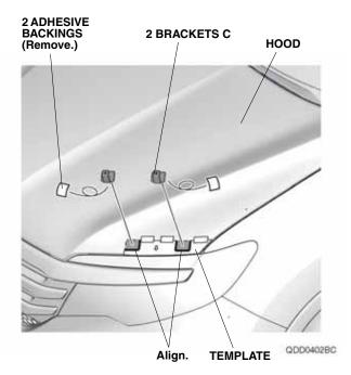
8. Turn the template over and repeat steps 5 through 7 to install the other two brackets C on the right side of the vehicle.
