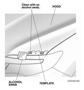
7. Remove the two adhesive backings from the two brackets C, and align them with the template secured in step 5. Remove the template.
