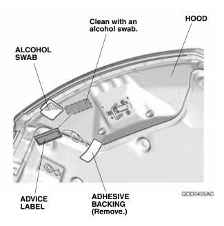
Remove the adhesive backing from the advice label, and attach the advice label to the hood as shown.
