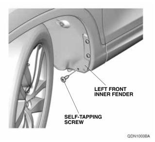
4. Loosely secure the left front splash guard on the left front inner fender with two 5 x 20 mm self-tapping screws and the self-tapping screw removed in step 3.
