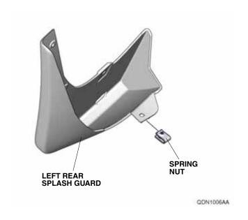
9. Install one spring nut on the left rear inner fender through the hole shown.
