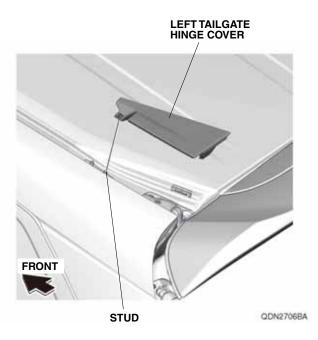
6. Open the tailgate. Reinstall the left tailgate hinge cover extension on the left tailgate hinge cover with one clip and one pin.
