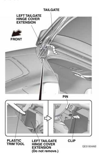
3. Close the tailgate halfway. Gently pry up on the rear edge of the left tailgate hinge cover. Discard the left tailgate hinge cover.
