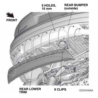
Secure the rear lower trim with nine clips A. NOTE: Do not push the clip too tightly, or it may deform the rear lower trim. Readjust the clip, if necessary.
