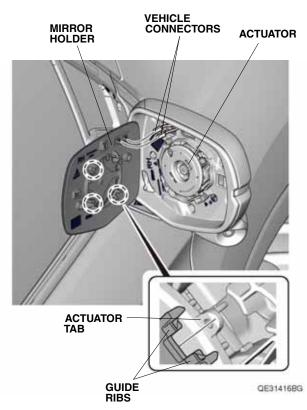
14. Align the guide ribs on the mirror holder so they line up on each side with the actuator tabs. Reinstall the mirror holder on the actuator.
