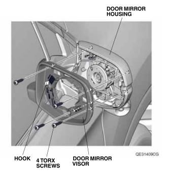
5. Using needle nose pliers wrapped with tape, remove the door mirror housing, and unplug the vehicle connectors.
