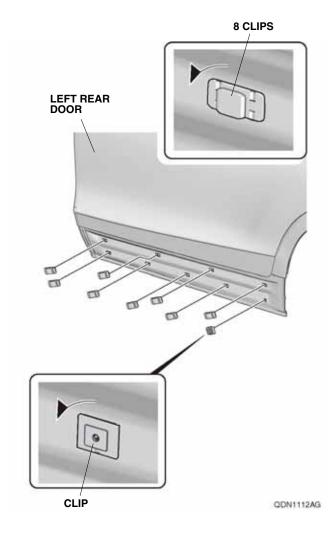
17. Reinstall the nine clips removed in step 16 and the screw removed in step 14 to the left rear door lower trim.
