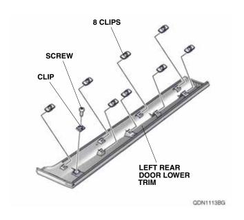
18. Attach the masking tape to the left rear door lower trim as shown.
