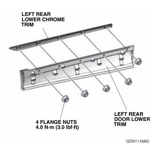
23. Secure the left rear lower chrome trim to the left rear door lower trim with five flange nuts. Torque the flange nut to 4.0 N·m (3.0 lbf·ft)
