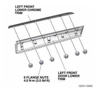
10. Secure the left front lower chrome trim to the left front door lower trim with six flange nuts. Torque the flange nut to 4.0 N·m (3.0 lbf·ft)
