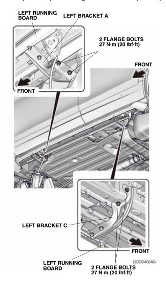
14. Align the green tape on the left running board harness with the hole on the left bracket A, and secure the left running board harness to the left bracket A with one wire tie.
