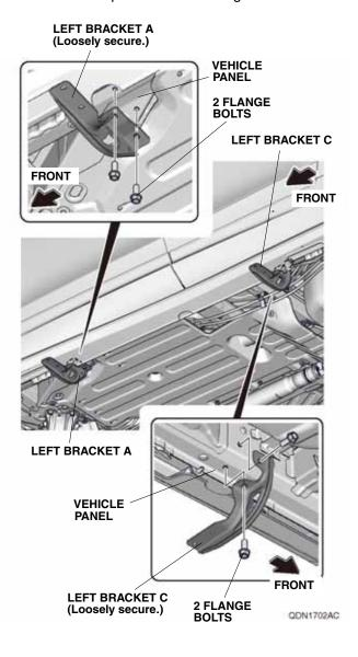
12. Secure the left running board to the left bracket A and left bracket C with four flange bolts. Torque the flange bolts to 27 N·m ( 20 lbf·ft).
