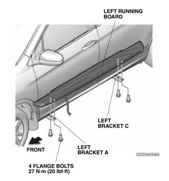
13. Tighten the four flange bolts loosely installed in step 11. Torque the flange bolts to 27 N·m (20 lbf·ft).
