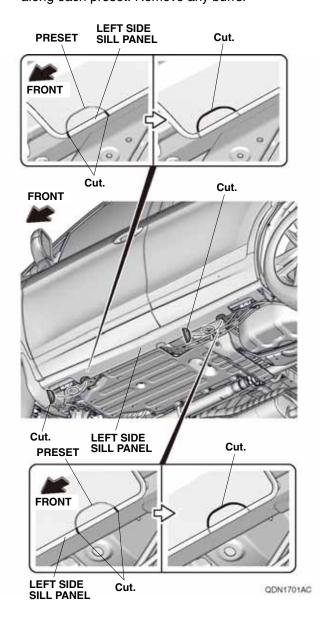
Remove the undercoating in the areas shown. Apply touch-up paint to the areas where you removed the undercoating, and allow them to dry thoroughly.
