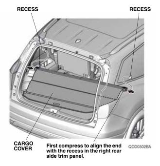
4. Attach each hook of the cargo cover to the headrestraint stay.
