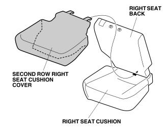
15. Attach the two hooks under the right seat cushion cover as shown.
