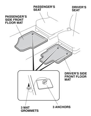
2. Install the passenger's side front floor mat by placing the mat grommet over the anchor on the floor carpet.
