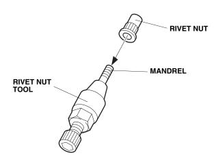
Insert the rivet nut into the hole in the vehicle frame and install the hex wrench on the rivet nut tool.
