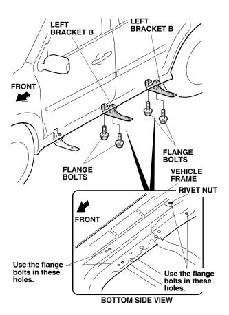
4. Position the left side step on the left bracket A and two left brackets B. Install the left side step with six flange bolts. Torque the flange bolts to 27 N·m (19 lbf·ft).
