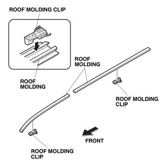
11. Reinstall the roof molding left cover.
