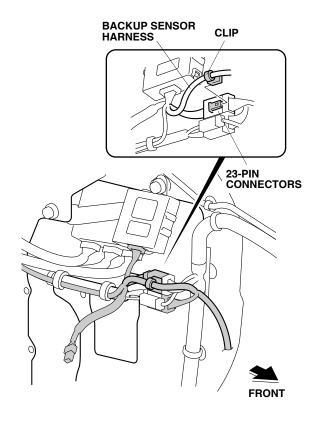
Route the backup sensor harness along the vehicle harness, and secure it to the vehicle harness with three wire ties.
