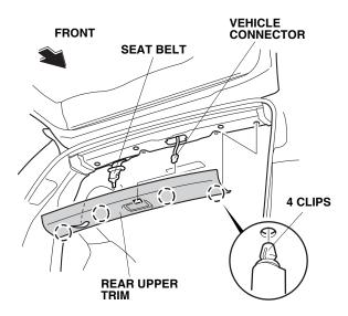
7. Use a small flat-tip screwdriver to push on the buckle to release each seat belt lower hook from the left third row seat.
