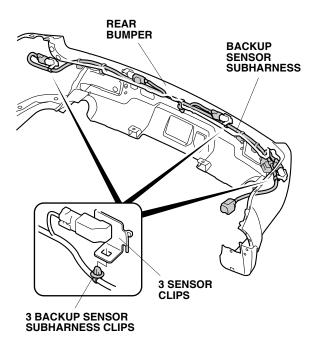
63. Secure the four backup sensor subharness clips to the four ribs on the rear bumper as shown.
