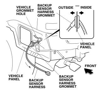
44. Slide the connector clip onto the backup sensor harness 6-pin connector, then install the connector clip into the vehicle panel hole.
