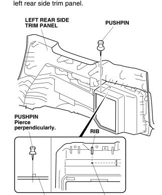
49. While wearing eye protection, drill a 3 mm hole at the pierced mark. Enlarge the 3 mm hole to 26 mm using a 26 mm hole saw. NOTE: Make sure to drill perpendicularly to the left rear side trim panel.
