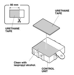
24. Using scissors, cut one urethane tape at the measurement shown. Attach the cut urethane tape to the control unit in the area shown.
