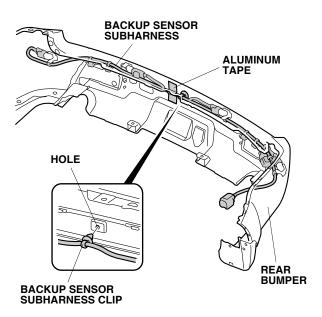
65. Using isopropyl alcohol on a shop towel, clean the rear bumper where the aluminum tape will attach. Secure the backup sensor subharness to the rear bumper with one aluminum tape.
