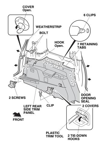
14. Pull away the weatherstrip and door opening seal at the front and rear of the left rear side trim panel.
