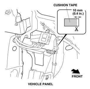
31. Using isopropyl alcohol on a shop towel, clean the vehicle panel where the cushion tape will attach. Attach the cushion tape to the vehicle panel in the area shown. 32. Plug the backup sensor harness 14-pin connector into the control unit.
