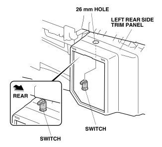
51. Using isopropyl alcohol on a shop towel, clean the switch bracket where the cushion tape will attach. Attach the remaining piece of cushion tape (from step 30) to the switch bracket as shown.
