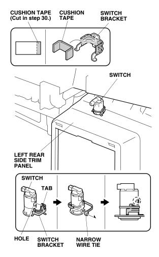
52. Secure the switch bracket to the switch using the narrow wire tie.
