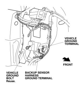
41. Route the backup sensor harness along the vehicle harness, and secure it to the vehicle harness with three wire ties.
