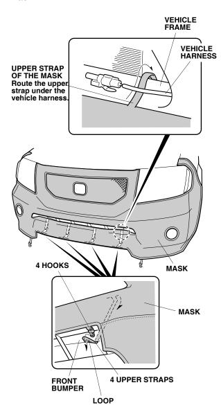
10. Attach the two plastic hooks to the bottom inside edge of the front bumper as shown.
